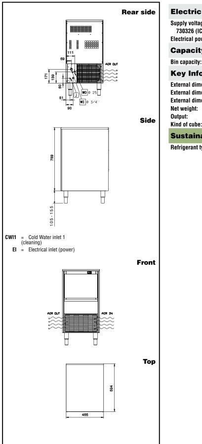
Supply voltage: 730326 (ICC37I20SNP) 220-240 V/1N ph/50 Hz **Electrical power max.:** 0.38 kW **Capacity:** Bin capacity: 20 kg **Key Information:** External dimensions, Width: 465 mm External dimensions, Depth: 595 mm External dimensions, Height: 894 mm Net weight: 45 kg Output: 37 kg/day Kind of cube: Ice Cube 22 g **Sustainability** R290 **Refrigerant type:**
